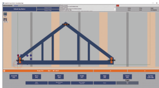
Iris™ Truss Software showing roof truss
